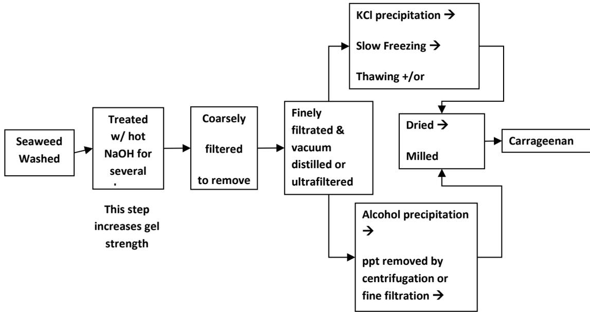
Figure 1: The general, non-proprietary production methods of Carrageenan (McHugh, 2003)
