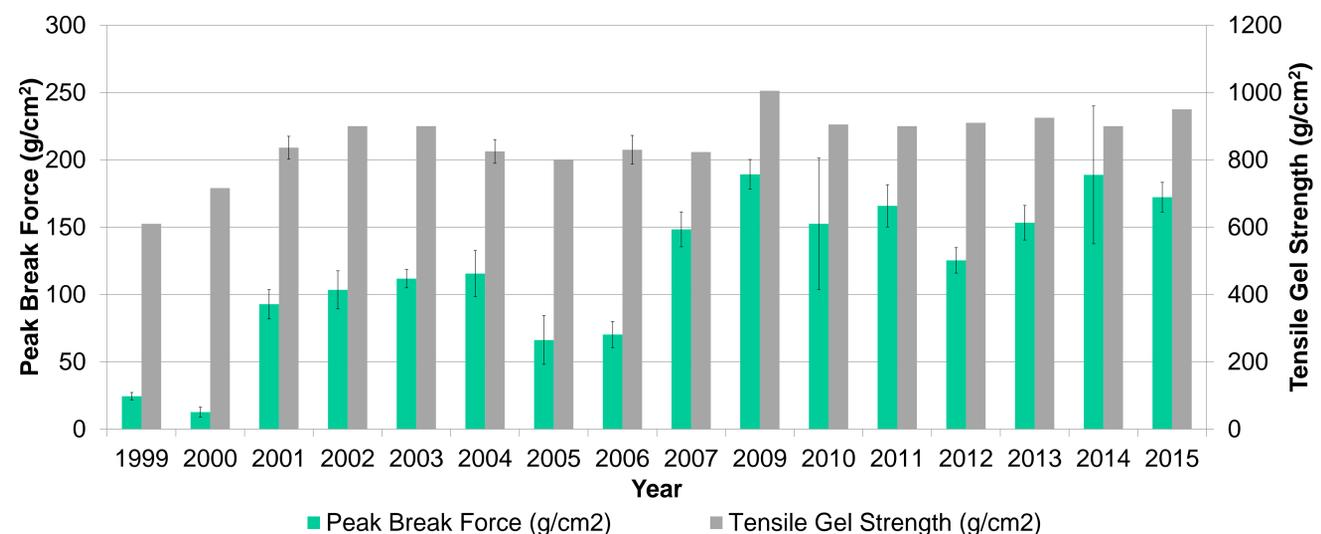
**Figure 2.** Comparison of average peak break force (g/cm<sup>2</sup>) and tensile gel strength (g/cm<sup>2</sup>) for 0.6% Agar from *Gelidium* sp (Product No. A296). Error bars are +/- one standard deviation.
