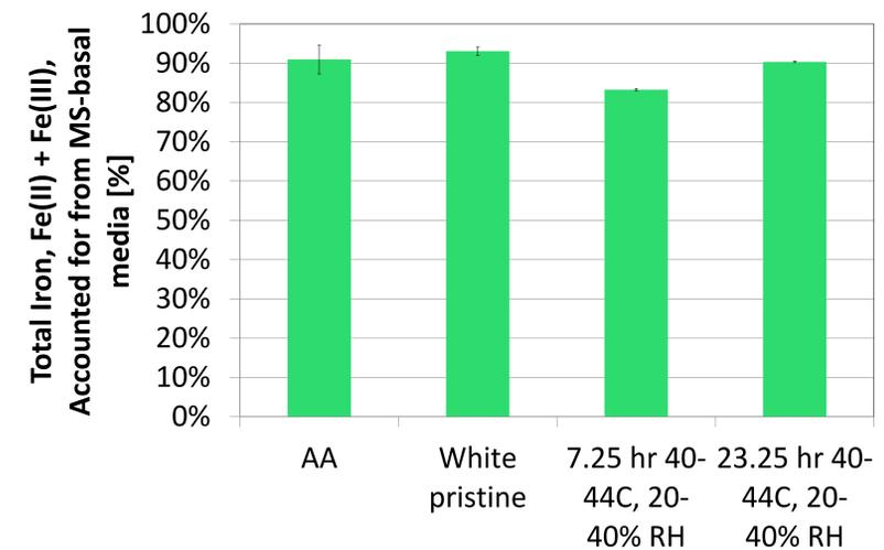
**Figure 4.** Recovered iron content, Fe(II)+Fe(III) as a percent of total iron content in MS basal media after dissolution
