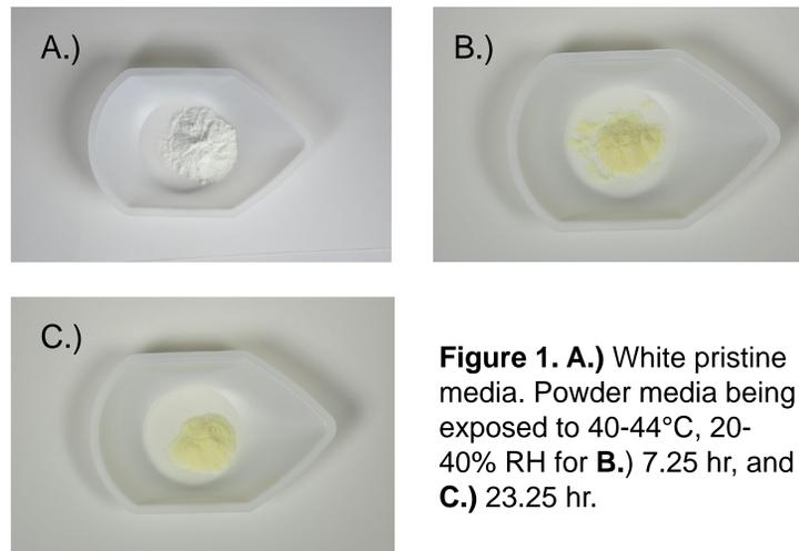
**Figure 1. A.)** White pristine media. Powder media being exposed to 40-44°C, 20-40% RH for **B.)** 7.25 hr, and **C.)** 23.25 hr.
